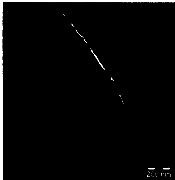
Figure 3-25: TEM nickel-coated HNTs
